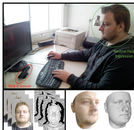
Figure 1: Hardware Setup: The RGB-D stream of a single PrimeSense Carmine is used to reconstruct high-quality head models using an interactive and intuitive reconstruction paradigm.
