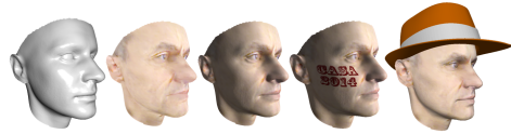
Figure 10: Applications: The textured models can be relighted, retextured and used for virtual try-on.
