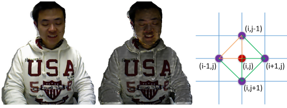
Figure 3: Left: Albedo estimation. input image and estimated albedo map. Right: spatial neighborhood of geometric regularizer.
