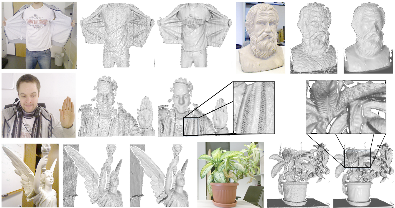
Figure 12: From a raw depth map and an aligned RGB image, our approach generates rich details on real-world data. Our method captures far more details than the raw depth map on static scenes, i.e., Socrates sequence, Lucy sequence and Flower sequence. Besides, our per-frame refinement method can be readily applied to dynamic scenes, e.g. human performances, as shown on Body sequence and Upper Body sequence. The closeup of the scarf region demonstrates the amount of small-scale detail captured by our method.
