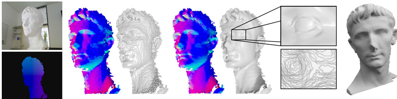
Figure 1: Our method takes as input depth and aligned RGB images from any consumer depth camera (here a PrimeSense Carmine 1.09). Per-frame and in real-time we approximate the incident lighting and albedo, and use these for geometry refinement. From left: Example input depth and RGB image; raw depth input prior to refinement (rendered with normals and phong shading, respectively); our refined result, note detail on the eye (top right) compared to original depth map (bottom right); full 3D reconstruction using our refined depth maps in the real-time scan integration method of [Nießner et al. 2013] (far right)
