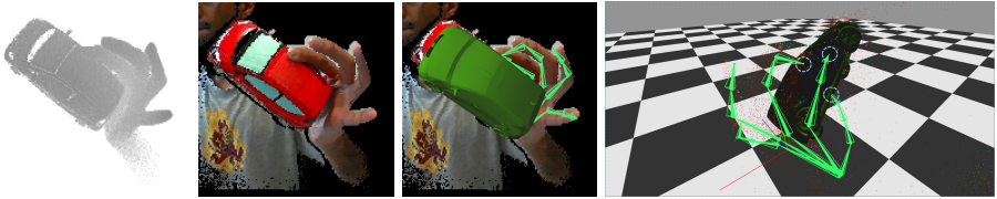
Fig. 2. We are able to track complex shapes like a toy car. Our contact points term (contacts are circled in blue) makes fingers hold the car even in the presence of severe occlusion.
