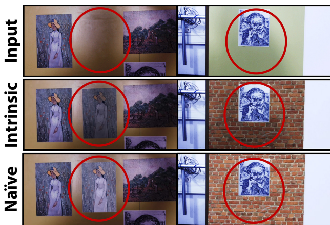
Figure 16: Realistic texture replacement: we add a virtual painting (left), and apply a brick texture (right). The textures realistically interact with the illumination (red circles). With a naïve texturing approach, shadows are lost. See this result in motion in our video.
