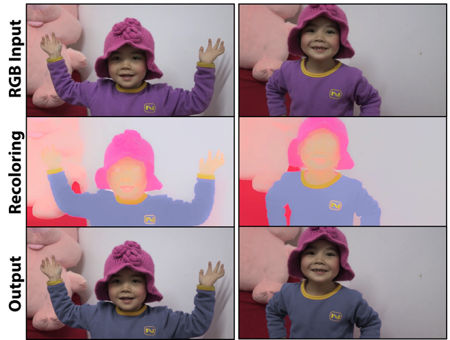
Figure 14: Reflectance recoloring on the GIRL sequence. We recolor the girl’s shirt in real time using our intrinsic decomposition approach. Note that the shading detail is preserved.
