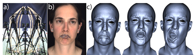
Figure 3: High-Quality Lip Database - Using a controlled multi-view capture setup (a), and lip tattoos (b), we reconstruct high-quality lip shapes for training (c).
